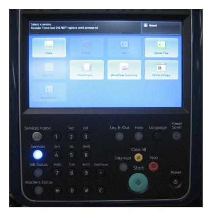
The control panel, which can be tilted and swivels left or back to the original position, has hard keys, including an alphanumeric keypad, and some LEDs (of note, one for when the unit is in sleep mode). The Help function offers guidance with specific jobs and, BLI technicians think, provides a high level of support. Users can check consumables levels by pressing the Machine Status hard key and then the Supplies tab. (U.S. model pictured)
