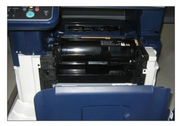
Replacing toner is clean. Users must first turn the control panel to the left and can then open the front cover, which includes most of the output tray; the black tabs on the cartridge must be unlocked, after which users can simply pull out the cartridge. Instructions on the touchscreen and the packaging provide guidance, should it be needed. (U.S. model pictured)
